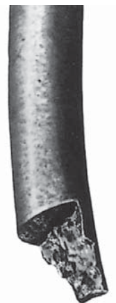
Example of fatigue failure
